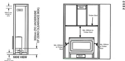
MUST USE NON-COMBUSTIBLE MA-TERIALS 315MM ABOVE THE UNITS OUTER SHELL(REDUCED CLEAR-ANCE BOX), 200MM FROM THE SIDES OF THE OUTER SHELL AND ALL BELOW THE HEATER.
